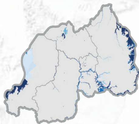
Flood hazard map for 1 in a 100 years probability evaluated under current climate conditions, the scale of blues represents different water depth values.
