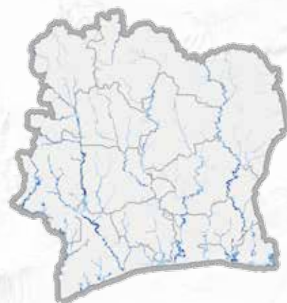
Flood hazard map for 1 in a 100 years probability evaluated under current climate conditions, the scale of blues represents different water depth values.
