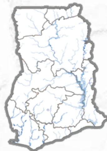
Flood hazard map for 1 in a 100 years probability evaluated under current climate conditions, the scale of blues represents different water depth values.
