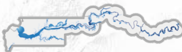
Flood hazard map for 1 in a 100 years probability evaluated under current climate conditions, the scale of blues represents different water depth values.
